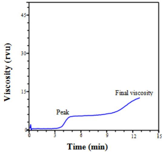
Figure 1c. Viscosity of spontaneously fermented maize meal (fermentation time = 24 h)
